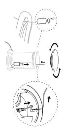
Unscrew frame cap opposite to the coaxial cable. Hook the cable gripper into the pocket inside the frame and guide the cable through the u-shaped hook in the
