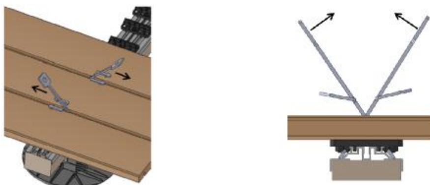
Picture 13: top left : the keys are driven simultaneously. Figure 18: top right , the action creates the detachment of the clips from the substructure without compromising the integrity of these (photo Grad TM )
